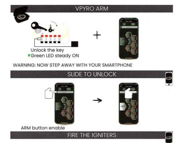
Keep pressed ARM button and ignite each single output with FIRE button. Or ignite all outputs togheter activating FIRE ALL button from App setting menu.
